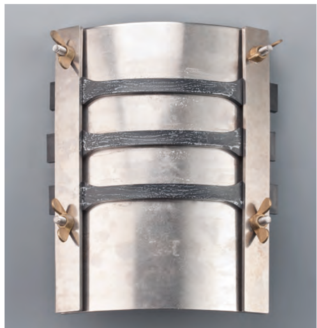
Figure 5: Stress crack resistance test by means of the bent strip method, conducted analogously to DIN EN ISO 22088-3; Ultradur ® B4300 G6 bk 5110 on the left and Ultradur ® B4330 G6 HR bk 15045 on the right.
