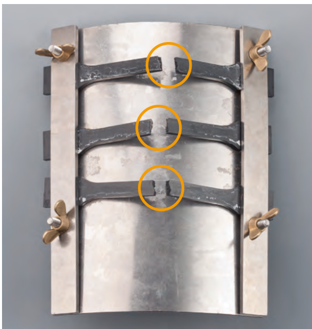
Figure 5: Stress crack resistance test by means of the bent strip method, conducted analogously to DIN EN ISO 22088-3; Ultradur ® B4300 G6 bk 5110 on the left and Ultradur ® B4330 G6 HR bk 15045 on the right.
