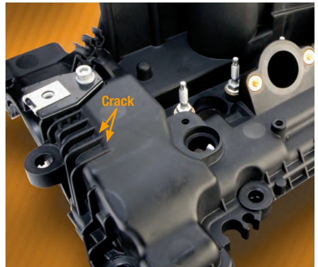
Figure 4: Visible surface damage after short-term contact with sulfuric acid (2%).
