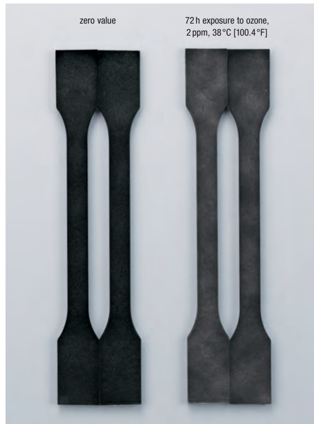
Figure 56: Test specimens made of Ultramid ® TKR 4355 G7 bk 564 before and after exposure to ozone. The color of the test bars faded slightly due to ozone exposure but the material properties remained largely unchanged.
